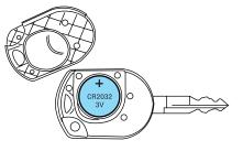
2. Do not wipe off any grease on the battery terminals on the back surface of the circuit board.
